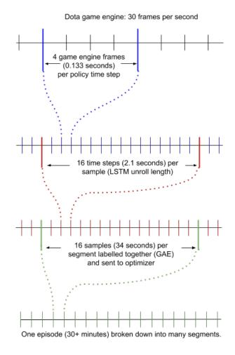
Figure 8: **Timescales and Staleness:** The breakdown of a rollout game. Rather than collect an entire game before sending it to the optimizers, rollout machines send data in shorter segments. The segment is further subdivided into samples of 16 policy actions which are optimized together using truncated BPTT. Each policy action bundles together four game engine frames.
