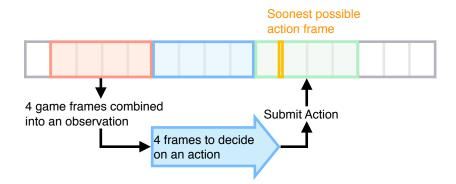
Figure 19: **Reaction Time:** OpenAI Five observes four frames bundled together, so any surprising new information will become available at a random frame in the red region. The model then processes the observation in parallel while the game engine runs forward four more frames. The soonest it can submit an action based on the red observations is marked in yellow. This is between 5 and 8 frames (167-267ms) after the surprising event.
